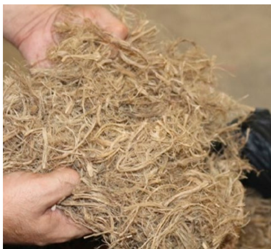
Fig. 1. Kenaf fiber (cut 30 mm length)
