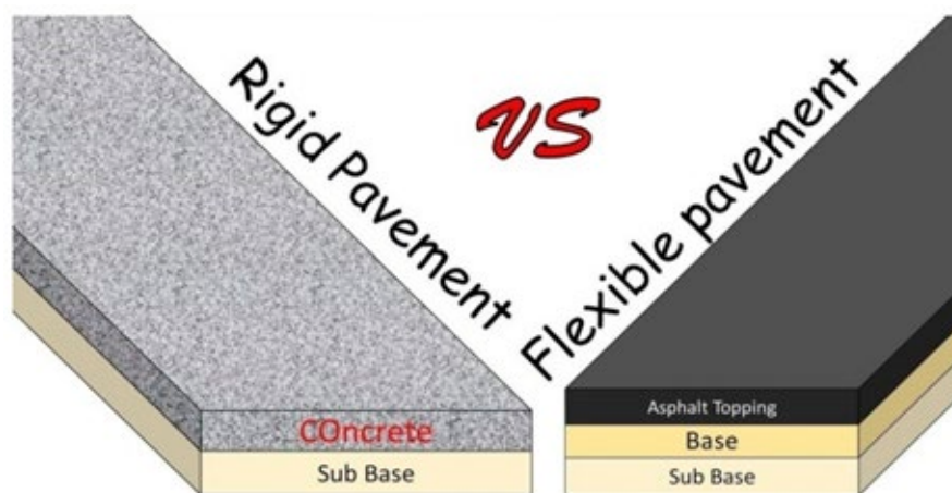
Figure 2. Flexible Pavement Vs Rigid Payment Layers
